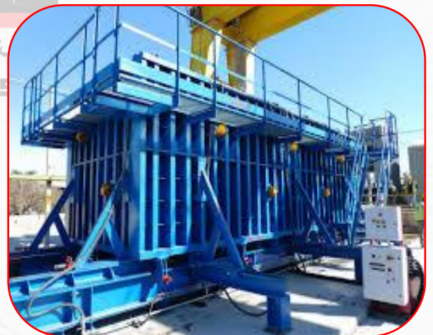
Precast Steel Mould
